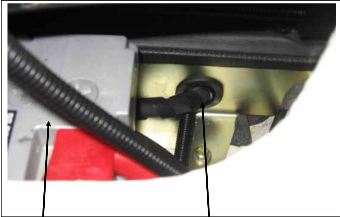
13/32" hose and clutch wire passing through existing grommet
