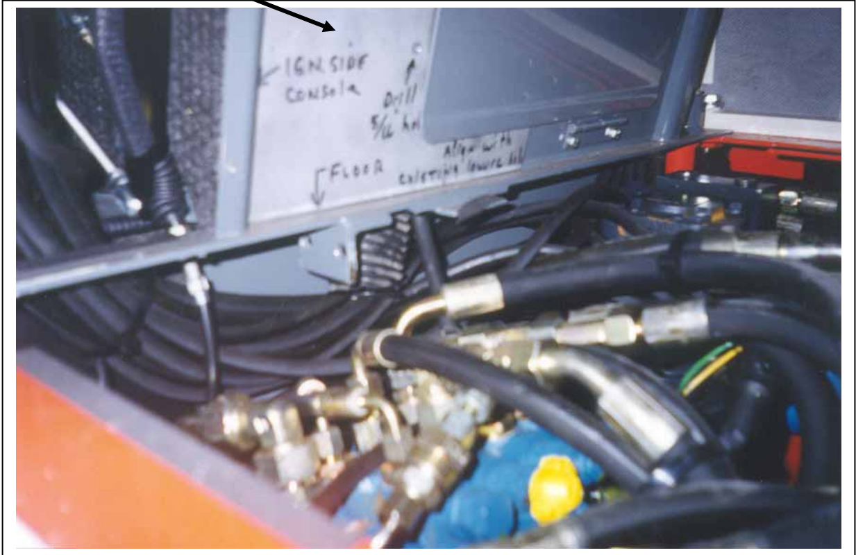
Front mounting hole template in place
