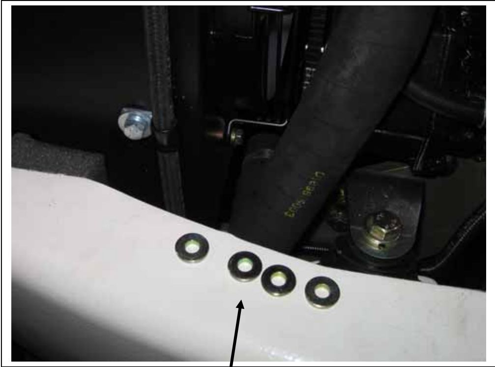
Four washers removed from the fan screen.
