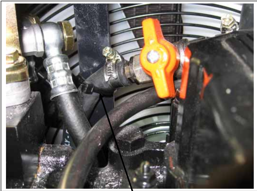
Tie the heater hose to the compressor mount stiffener bracket.
