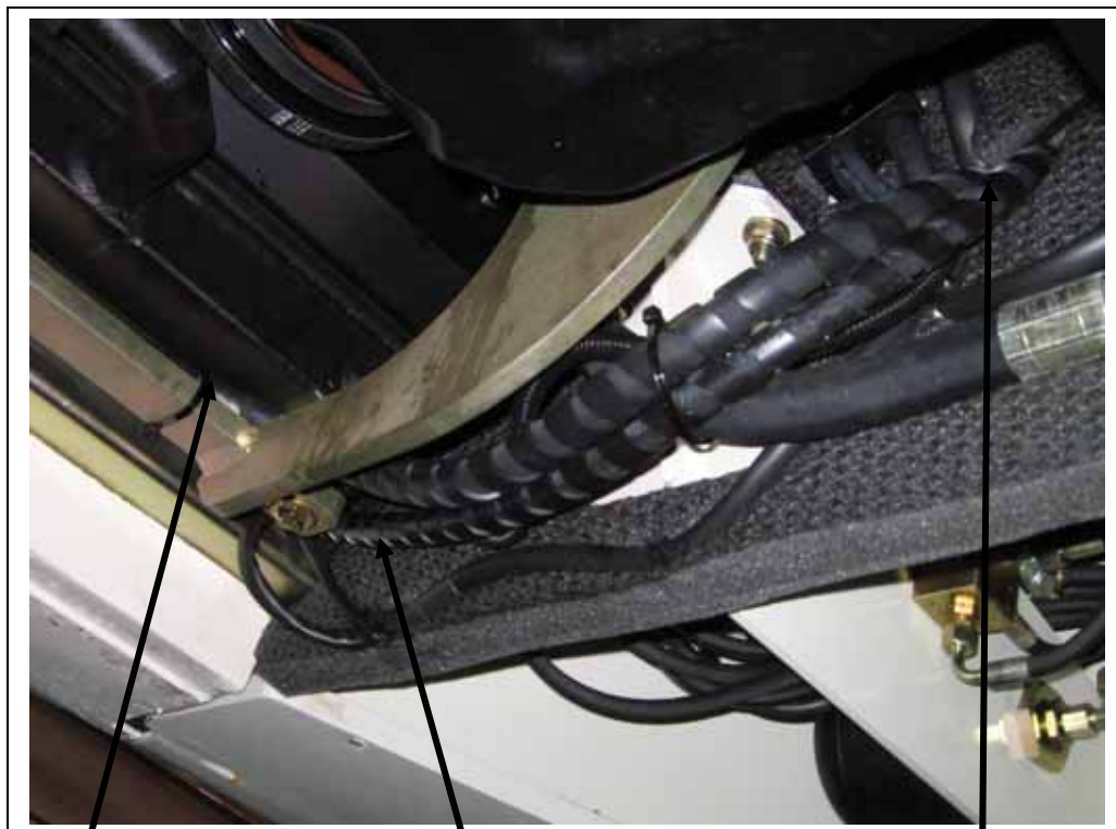
1/2" line on radiator support frame
