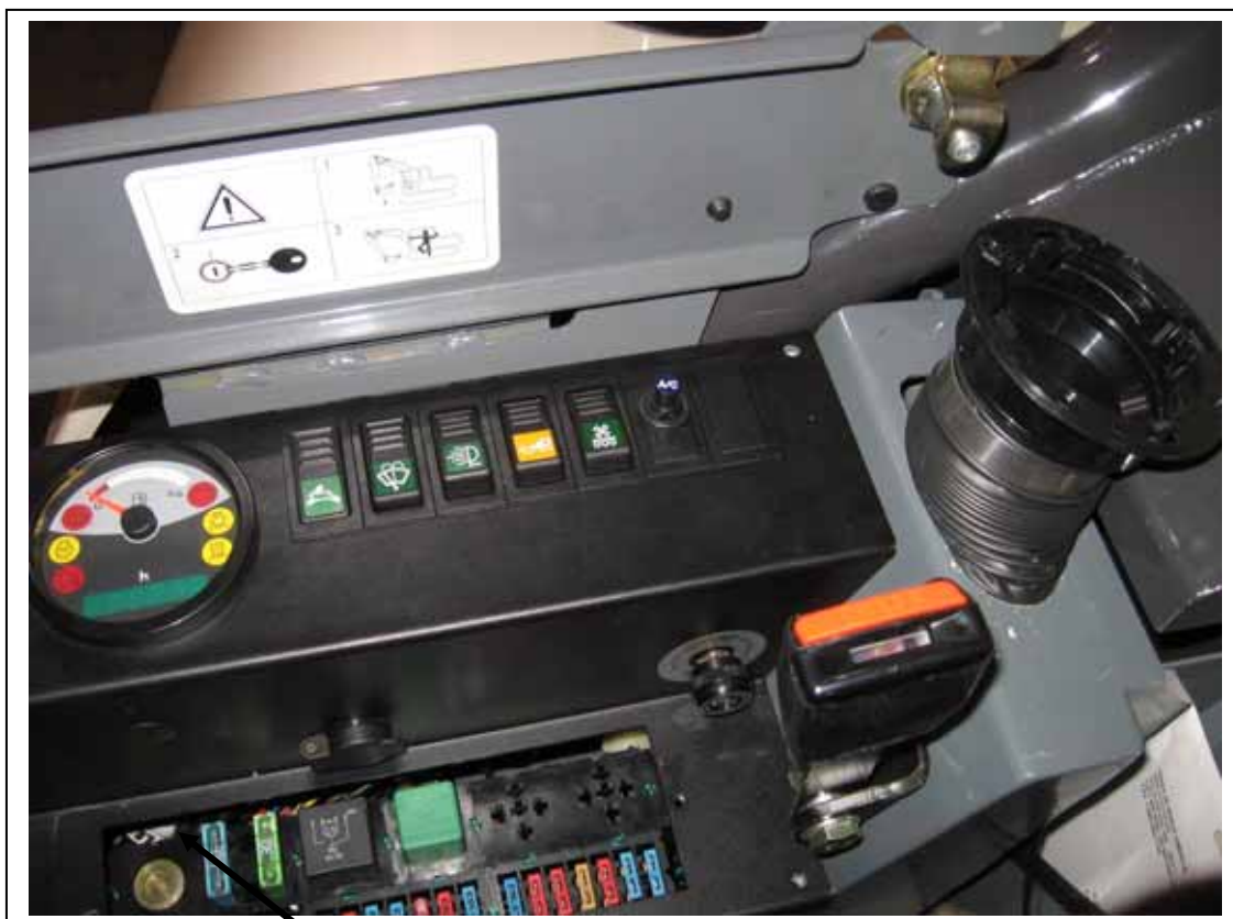
Ignition live power wire found down beside the fuse panel. Access by lifting up control panel.
